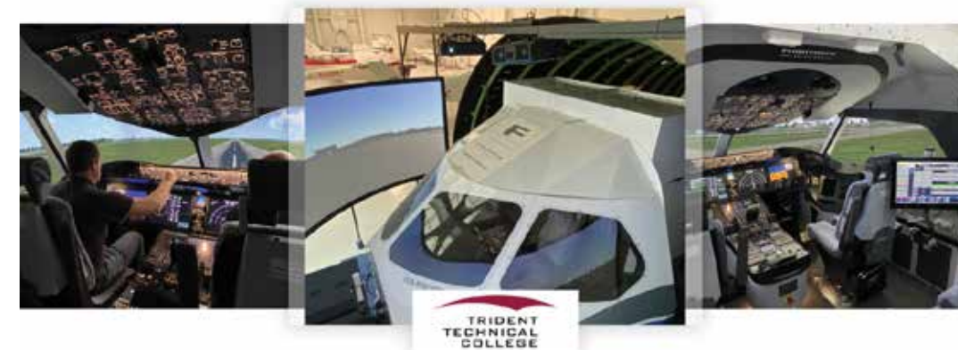
FDS-B787-FTD device at Trident Technical College, Charleston, SC, USA.
